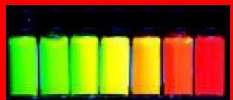
CdTe hydrophilic Q-dots are coated with -COOH groups and can be easily used for labeling purposes for chemical and biological applications.
